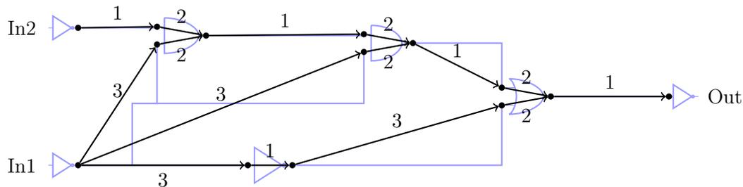
The edge labels specify the delays. We do not distinguish between rising and falling signals and do not consider slew. Maximum (late mode) and minimum (early mode) delays are equal. Assume that all the arrival times for the latest and earliest signal at the primary inputs 'In1' and 'In2' are 0 and the required arrival times at the primary output 'Out' are 10 (early mode) and 12 (late mode).
