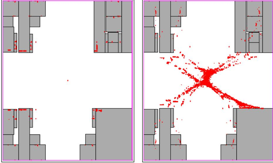
**Figure 9.** Minimizing the linear bounding box net length (left) gives hardly any information on relative positions compared to minimizing quadratic net length (right). As no disjointness constraints were considered yet, many cells share their position, especially on the left-hand side.
