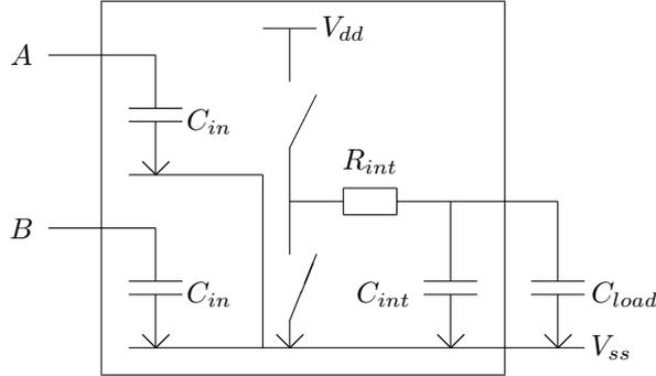
**Figure 19.** A simple electrical model of a circuit. The input capacitance  $C_{in}$  and the internal capacitance  $C_{int}$  are proportional to the scaling factor of the circuit while the internal resistance  $R_{int}$  is antiproportional.
