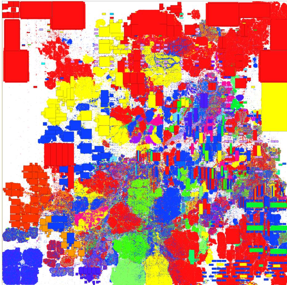
**Figure 30.** A system on a chip designed in 2006 with BonnTools. This 90nm design for a forthcoming IBM server has more than 5 million circuits and runs with frequencies up to 1.5 GHz. Colors reflect the structure of the underlying logic blocks.
