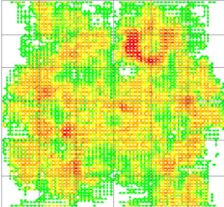
**Figure 28.** A typical global routing congestion map. Each edge corresponds to approximately 10x10 global routing edges (and to approximately 1 000 detailed routing channels). Red, orange, yellow, green, and white edges correspond to an average load of approximately 90–100%, 70–90%, 60–70%, 40–60%, and less than 40%.
