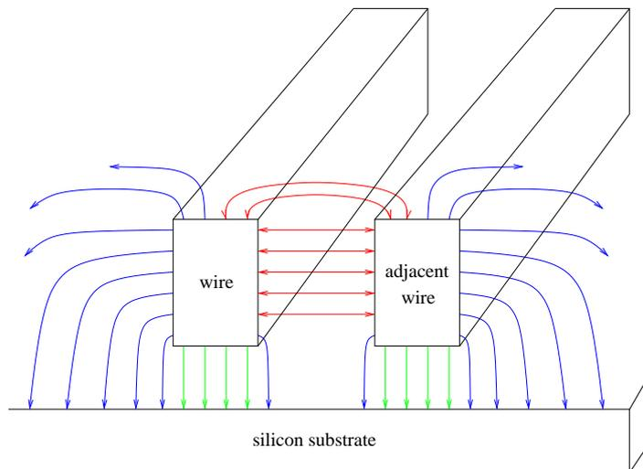
**Figure 27.** The capacitance of a net consists of area capacitance (green) between the undersurface of the wire and the substrate, proportional to length times width, fringing capacitance (blue) between side face of the wire and substrate, proportional to length, and coupling capacitance (red), proportional to length if adjacent wires exist. Note that the wire height is fixed within each plane, while the width varies.
