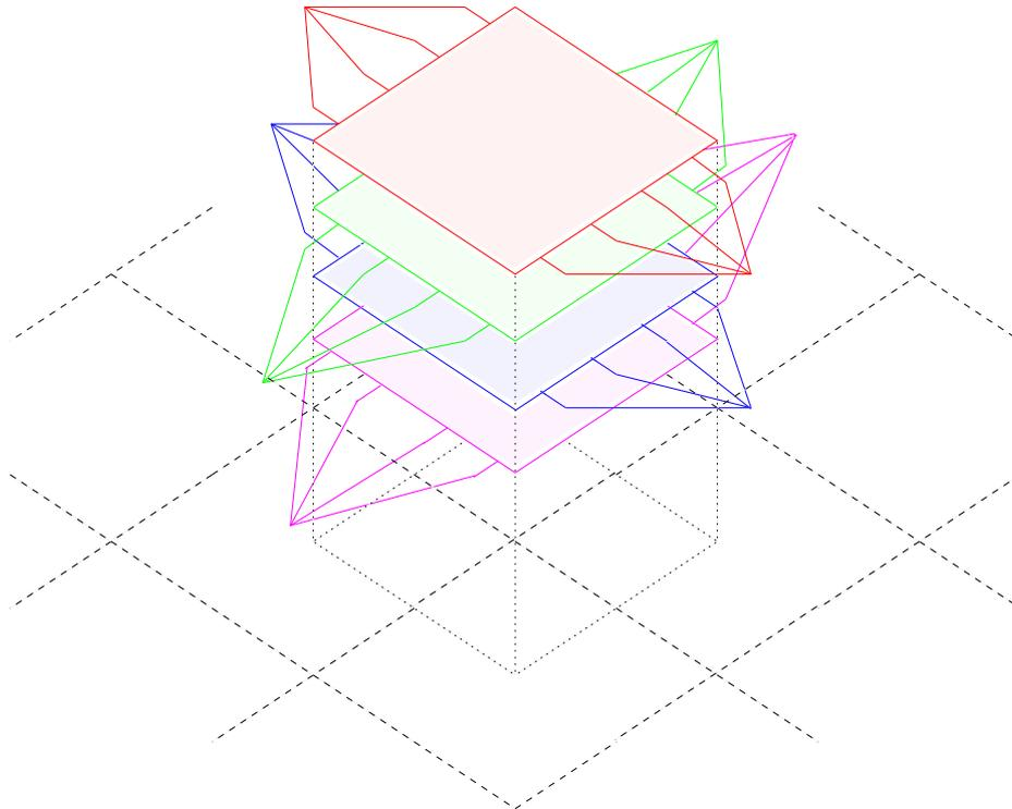
**Figure 26.** An instance of the vertex-disjoint paths problem for estimating global routing capacities. Dashed lines bound global routing regions. Here we show four wiring planes, each with a commodity (shown in different colors), in alternating preference directions.
