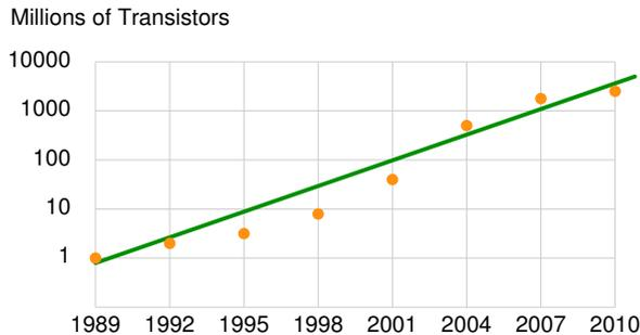
Figure 1. Number of transistors per logic chip
