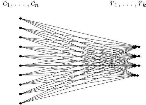
**Figure 10.** The Hitchcock transportation problem is a relaxation of the multisection problem. All arcs are oriented from left to right and are uncapacitated. The supply vertices on the left correspond to movable objects and have supply  $size(c_1), \dots, size(c_n)$ . The demand vertices on the right correspond to subregions and have demand  $cap(r_1), \dots, cap(r_k)$ . Arc costs are  $d(c_i, r_j)$  for all  $1 \leq i \leq n, 1 \leq j \leq k$ . Note that  $k \ll n$  in this application.
