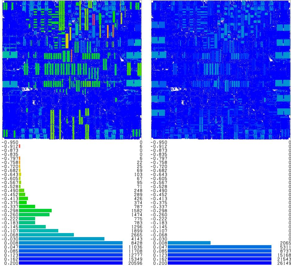
**Figure 22.** Slack histograms showing the improvement due to clock skew scheduling and appropriate clock tree synthesis; left: zero skew, right: with BonnClock trees. Each histogram row represents a slack interval (in ns) and shows the number of circuits with their worst slacks in this range. The placements on top are also colored according to the worst circuit slacks.
