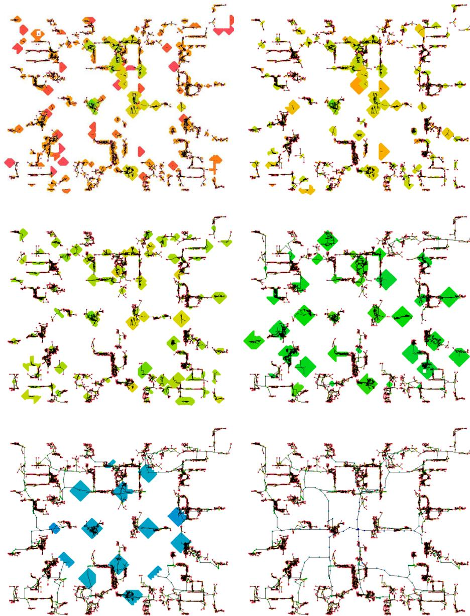
**Figure 23.** Different stages of a clock tree construction using BonnClock. The colored octagons indicate areas in which inverters (current sinks) can be placed. The colors correspond to arrival times within the clock tree: blue for signals close to the source, and green, yellow, and red for later arrival times. During the bottom-up construction the octagons slowly converge to the source, here located approximately at the center of the chip.
