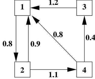
**Figure 21.** A latch graph with 4 latches (numbered boxes). The arc numbers specify the longest path delays. With a zero skew tree — when all latches switch simultaneously — the slowest path ( $3 \rightarrow 1$ ) determines the cycle time  $T_{zs} = 1.2$ . With an optimum scheduled tree the slowest average delay cycle ( $1 \rightarrow 2 \rightarrow 4 \rightarrow 1$ ) determines the cycle time  $T_{opt} = 0.9$ .
