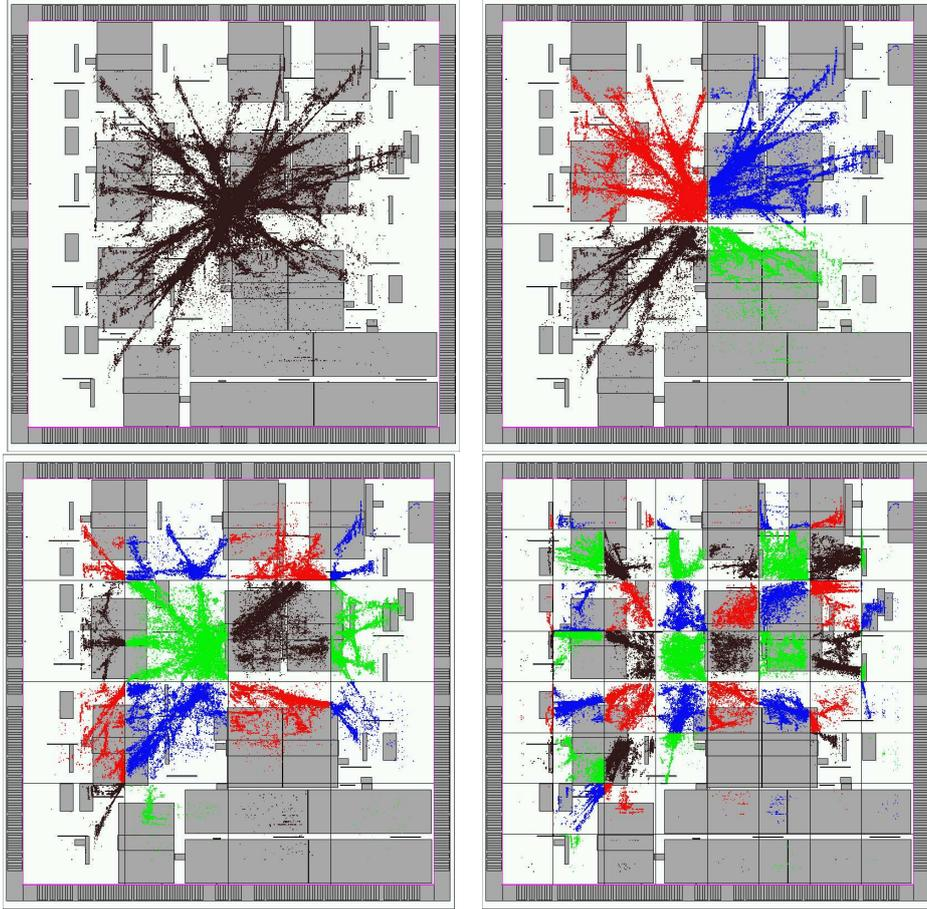
**Figure 8.** The initial four levels of the global placement with 1, 4, 16, and 64 regions. Colors indicate the assignment of the movable objects to the regions. The large grey objects are fixed and serve as blockages.
