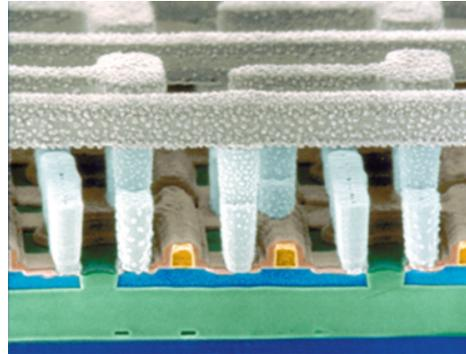
**Figure 5.** Microscopic view of a chip with aluminum wiring
