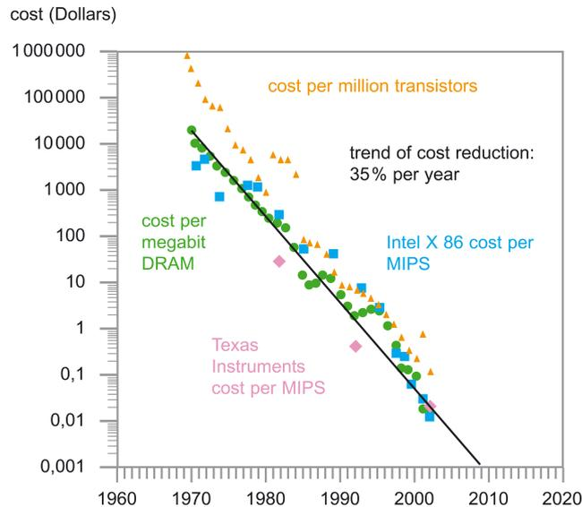
**Figure 3.** Trend of cost reduction in microelectronics
