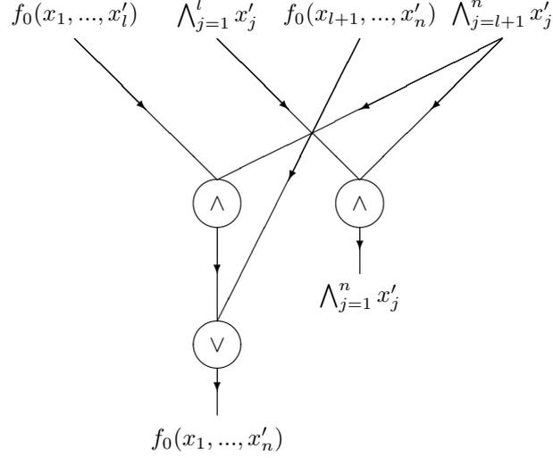
**Figure 18.** The logic circuit corresponding to equation (7)
