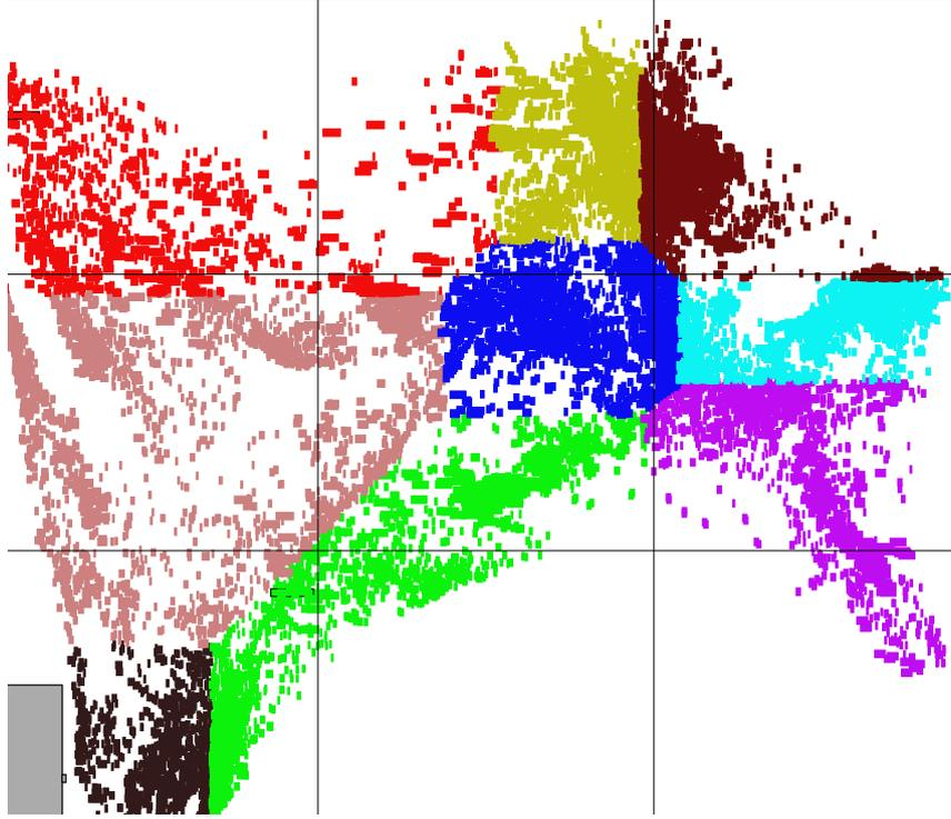
**Figure 11.** An example for multisection: objects are assigned to  $3 \times 3$  subregions. The colors reflect the assignment: the red objects are assigned to the top left region, the yellow ones to the top middle region, and so on. This assignment is optimal with respect to total  $\ell_1$ -distance.
