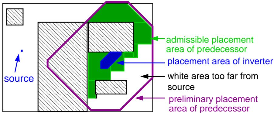
**Figure 24.** Computation of the feasible area for a predecessor of an inverter. From all points that are not too far away from the placement area of the inverter (blue) we subtract unusable areas (e.g., those blocked by macros) and points that are too far away from the source. The result (green) can again be represented as a union of octagons.
