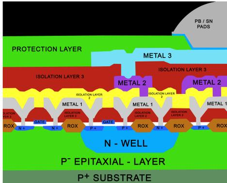
**Figure 4.** Schematic cross-sectional view of a chip
