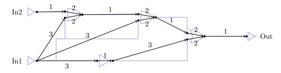
The edge labels specify the delays. We do not distinguish between rising and falling signals and do not consider slew. Maximum (late mode) and minimum (early mode) delays are equal. Assume that all the arrival times for the latest and earliest signal at the primary inputs 'In1' and 'In2' are 0 and the required arrival times at the primary output 'Out' are 10 (early mode) and 12 (late mode).
